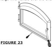
Twist the smaller wire handle over the end of the air damper rod below the door. Install ash pan pull handle using screws and washers. See FIGURE 26.
