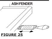
The draft can be adjusted from a low burn rate with the handle in fully, to a fast burn rate with the handle fully out. Inadequate draft may cause back-puffing into the room through the stove/insert and chimney connector points and may cause plugging of the chimney. Too much draft may cause an excessive temperature in the stove, glowing red stove parts or chimney connectors or an uncontrollable burn which can lead to a chimney fire or permanent damage to the unit.
